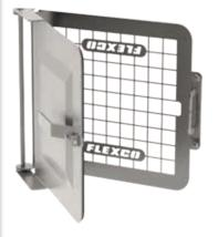
Chute Opening: 400 mm x 400 mm Outer Door: Solid c/w Lockable Handle Inner Mesh Door: 3 mm mesh @ 50 mm spacing Material: Grade 316 Stainless Steel Overall Weight: 13 kg
